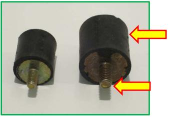
EDGE uses large and durable Isolators, which do the hard work on the machine. They are 1" diameter with 5/16" stud bolts. Shown next to alternative that is smaller in both areas. Many alternative isolators are also softer, which is required due to less powerful motors. Smaller/Softer isolators typically require more frequent replacement and can fail from impacts.
