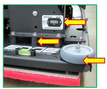
EDGE decks comes with a hour meter to track isolator time, for scheduled replacement every 1500 hours. An affordable kit includes new isolators, bolts, and a hour meter.
