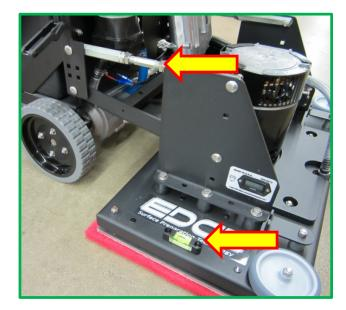
Steel Adjustment Rods (¾") and the standard levels allow the deck's alignment to be easily maintained. Proper alignment increases longevity of the pads and performance.
