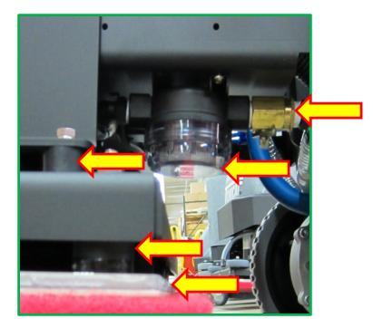
Oversized Solution Filter (stainless screen) and Brass gate valve for easy access and service.
