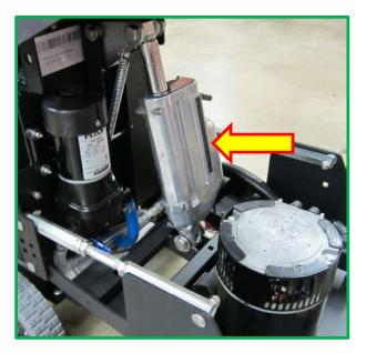
Powerful Actuator and HD Linkage handles the heavy scrub deck assembly. The onboard controller monitors pressure and the Manager Lockout Key (yellow) option gives oversight to performance.
