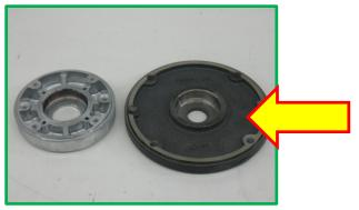
Our End Housing is cast iron (instead of softer aluminum) more securely locating the bottom bearing, which sees heavy loads from the oscillation.
