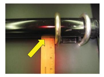
The GTX scrubber 2" axle is larger than axles on many other machines. The larger axle is designed to support the GTX scrubber in harsh applications and last the life of the machine.
