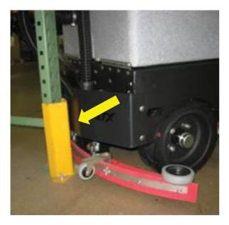
Our GTX scrubber comes standard with a heavy-duty steel rear bumper, which helps protect the squeegees in "reverse" collisions. All scrubbers offer "breakaway" squeegees for "forward" collisions.
