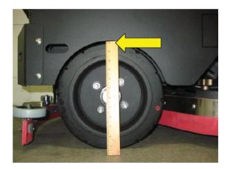
GTX scrubber's have a 12" diameter tire. The large diameter improves the ride over expansion joints and irregular concrete surfaces. Each tire is rated at 2,200 lbs, which is 3 times greater than the load with full tanks.
