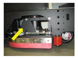
The GTX scrubber uses durable, heavy-duty steel trailing arms and scrub deck, which are better able to withstand collisions and be repaired in the field than machines with plastic trailing arms and cast aluminum scrub decks.
