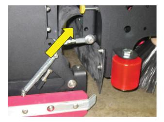
Unlike many other machines, the GTX scrubber has a barrier to stop water or debris from being thrown onto the scrub deck.
