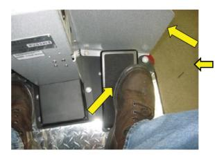
The GTX scrubber has a simple and large pedal, which controls speed. This view also shows the protection offered to the Operator's foot on the GTX scrubber. A complete apron across the front makes it harder for the operator to hang his foot off the side, reducing potential injuries.
