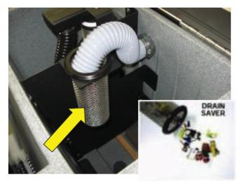
A feature to the GTX scrubber is the "Drain Saver" stainless steel basket that collects litter from recovery water. This reduces the potential of discharge water clogging the customer's floor drains. A simple device that can avoid costly drain repairs for customers.
