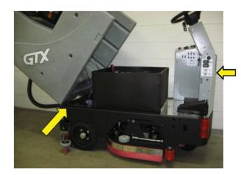
The GTX scrubber uses larger (8" stainless) hinges and bolt directly into the heavy gage steel frame. This provides better durability than other machines that use smaller tank hinges bolted to plastic tanks.
