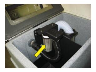
The GTX scrubber uses a stainless steel vacuum / foam protection screen, which can be cleaned and used for years, not like the less expensive plastic options. Our intent is that this will save the customer money.
